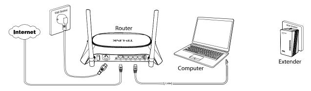
Figure 2-1 Hardware connection
